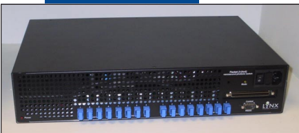
Lynx Photonic Networks' LightLEADER™ 3000 series are small optical communications systems—built around Lynx's patented intelligent optical switch fabrics
